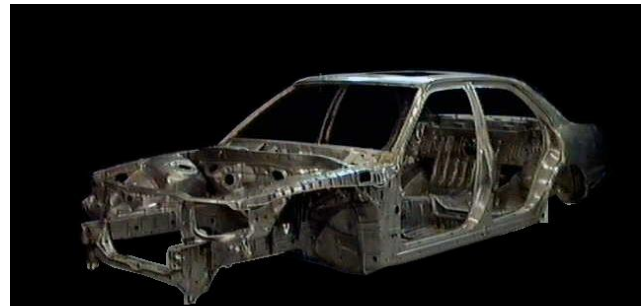
Figure 1. Body-in-white structure for a mid-sized car.
